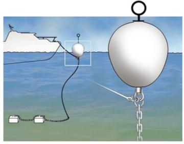
Do not expose the buoy to a load of more than 60% of its total buoyancy. Please also consider additional weight/load caused by marine growth, currents, wind and waves.
